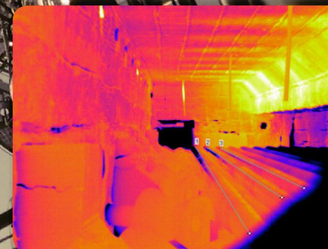
When thermal imaging inside refractory lined furnaces or boilers is required the plant operator is required to cut large openings in the refractory to enable viewing of the critical area. This can cause significant wasted energy from heat loss through the opening and can be difficult to keep the opening free from debris.
