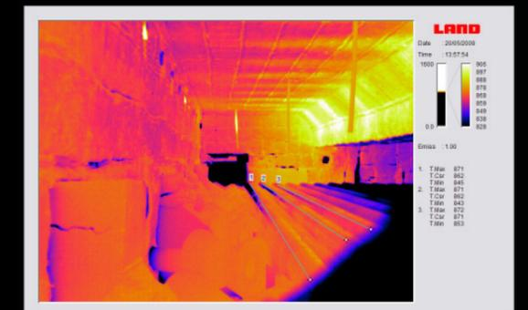
Temperature Profiles inside the furnace
