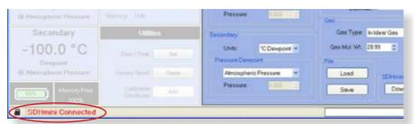
On your PC open the *SHAW SDHmini User Tool*. The view panel appears on the PC saying "SDHmini Connected".
