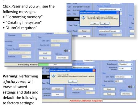
date format, language, main display units, secondary display, gas weight, gas type, AutoCal value and numerical delimiter.
