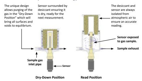
Keeping the sensor dry between tests ensures that the SDHmini is ready to carry out rapid spot checks. The unique design of the desiccant head achieves this by surrounding the sensor with desiccant, keeping the sensor dry. The head is then lifted for sampling, exposing the sensor to the sample gas.
