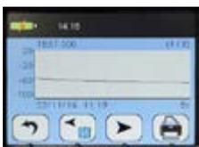
You will notice that the vertical red line cursor is missing and the corresponding measurement value is also missing from the top bar.
