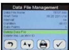
The *Data File Management* function allows the user to inspect how the data was captured and other file attributes. It also allows the possibility to delete the file and also ALL files associated with the *Location ID* but not the *Location ID* itself which will be saved ready for another logging event.
