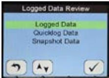
In order to inspect the files select the appropriate type of data by using
