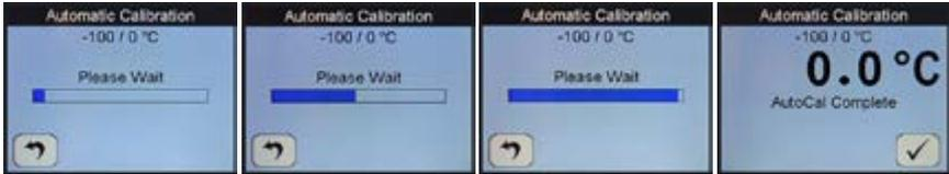
The SDHmini-L will now display the full scale value of the unit, either  $-20\text{ °C}$  or  $0\text{ °C}$  depending on the sensor range.
