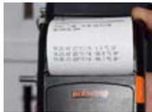
You may also print the data file using the printer icon key, provided as before, that the Bluetooth connection has been maintained or established.
