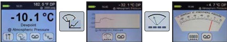
The digital display mode has the benefit of showing the moisture measurement in main choice of engineering units but also a secondary display with perhaps alternative engineering units. This mode also allows application of pressure dewpoint to evaluate the measurement in other samples pressures.
