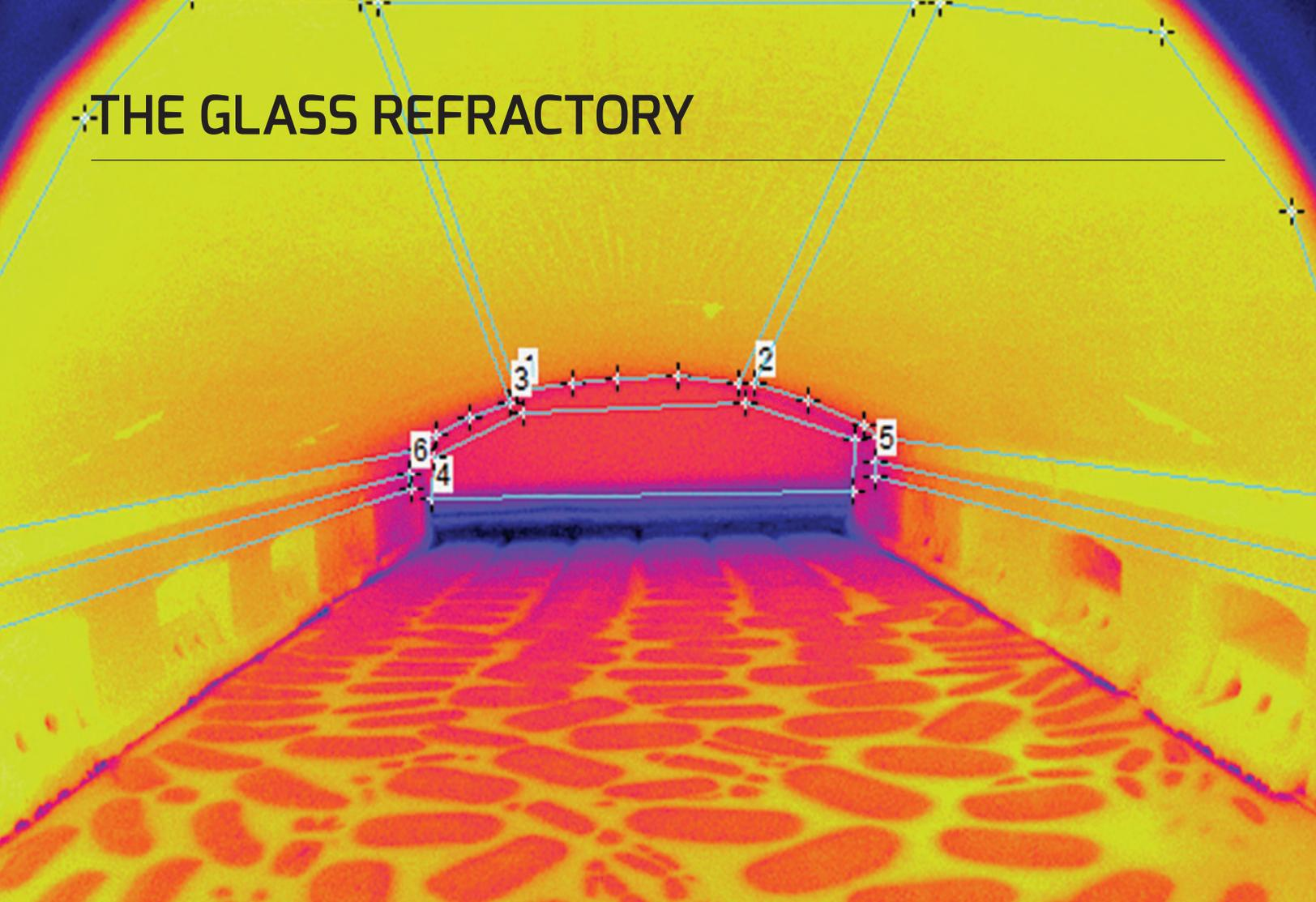
Nearly all glass production processes begin with raw materials being melted in a furnace or tank. Glass melting is highly energy-intensive, and takes place in continuously operated tanks. The process can take more than 24
