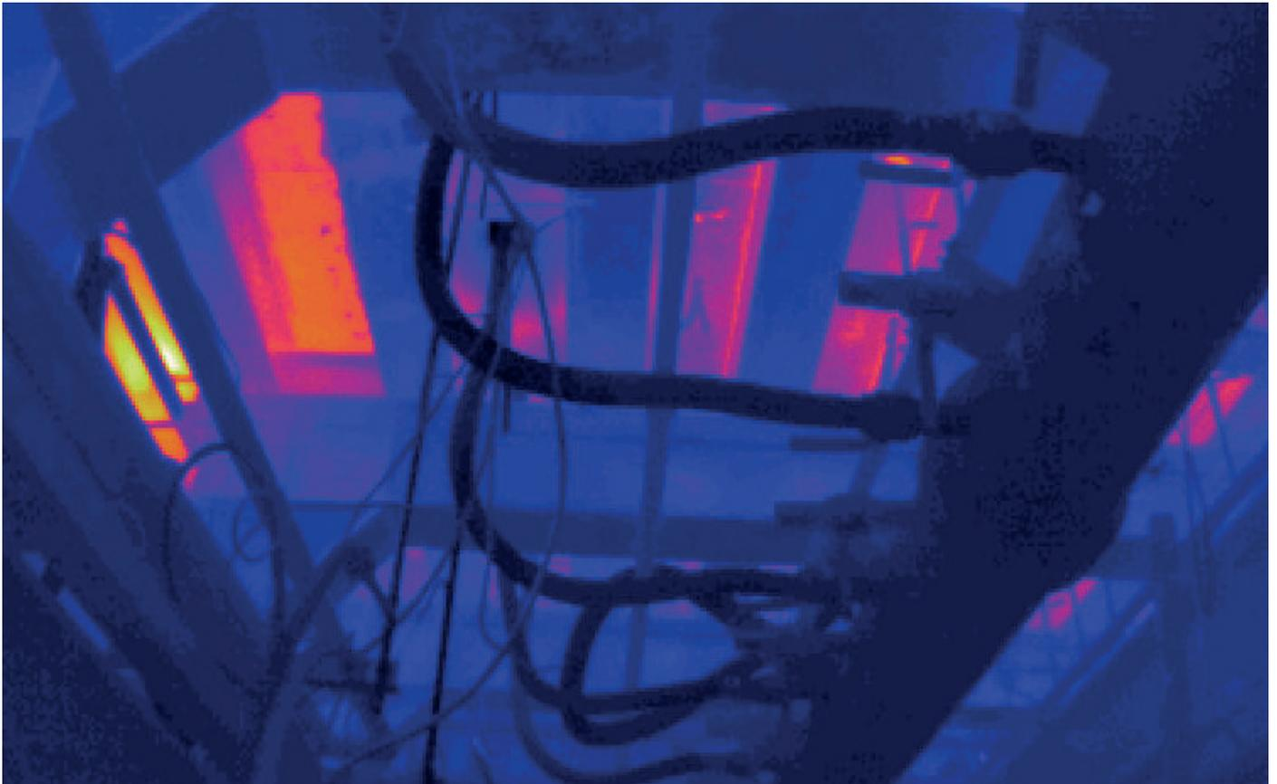
MONITORING OF TANK BOTTOM TEMPERATURES
