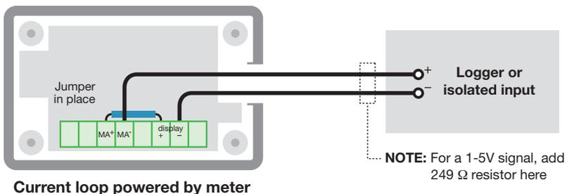
Current loop powered by meter
