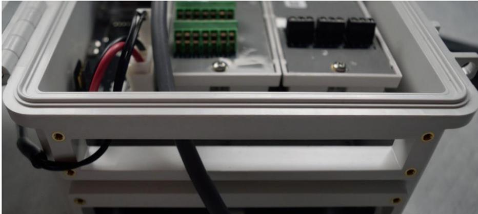
3. Insert one of the wires for the first parameter in the first available channel and screw it in tightly.
