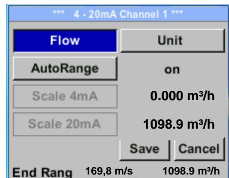
The 4-20 mA Analogue output of the Sensor VA 550 can be individually adjusted.
