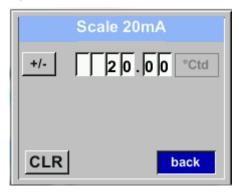
"Scale 4mA" and "Scale 20mA" allows defining the desired scaling.
