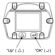
The operation of the FA 500 is done by the two capacitive key buttons Up ( $\triangle$ ) and Enter ( $\leftarrow$ )
