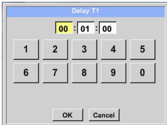
By changing the text field values the new delay time could be defined. Here for *Delay T1*.
