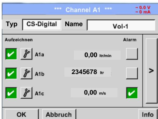
After the alarm activation at channel A1.
