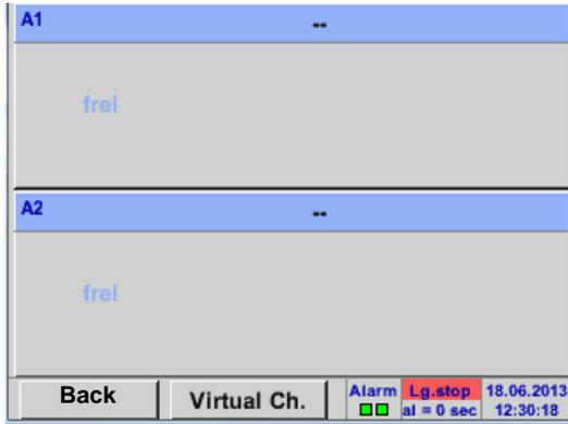
An overview of the available channels appears after entering the password. Depending on the version 2 or 4 channels.
