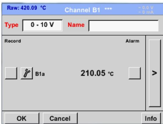
Please see the scale of the sensor (here for example *Type 0 - 10V* corresponds to 0 - 250 °C) from the data sheet of the connected sensor.
