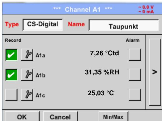
The DS 400 detects, if the connected sensor is a flow or dewpoint sensor of **CS Instruments** and set the *CS-Digital* subtype automatically correct.
