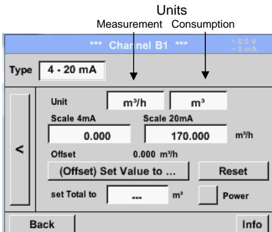
Selection of the units by pushing the text fields for the corresponding measurement and consumption units.
