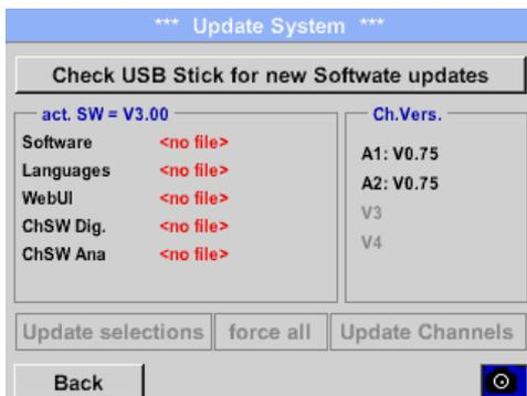
If after pressing the button "*Check USB Stick for new Software updates*" the following messages appear in the window, is the DS 400 is not properly connected to the USB flash drive or there are no files available.
