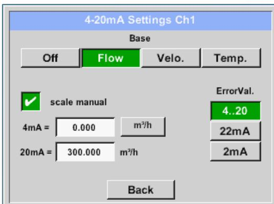
A "manual scaling" needs an activation of the "scale manual" button.
