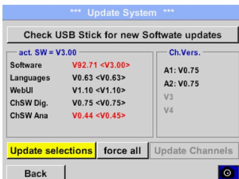
Is the DS 400 properly connected to the USB drive and there are new versions of the individual software parts available, then they are in red font and <new> marked.
