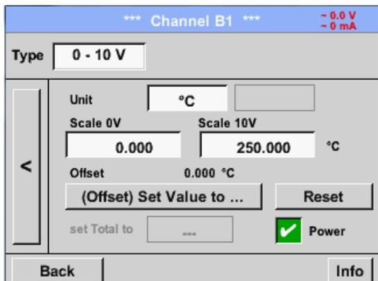
It is possible to define an Offset-Value. With the *Set Value to*-button (*Offset*) you enter it. The positive or negative difference of the *Offset* will be displayed.
