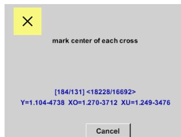
If necessary, the touch-screen calibration can be changed here. Push *Calibrate* and it appears, 1. left above, 2. bottom right, 3. bottom left, 4. right above and 5. in the middle, a calibration cross that must be pushed consecutively. If the calibration finished positive a message "*Calibration successful*" appears and have to be confirmed with *OK*. Is this not the case, so you can repeat the calibration with the help of the *Cancel* and *Calibrate* buttons.
