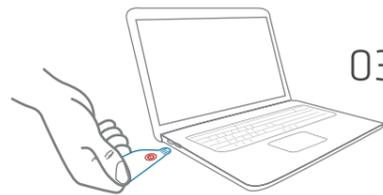
**03** Connect stopped logger directly to USB port
