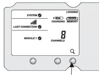
Press the Search button on the station again to stop the search for sensor nodes.
