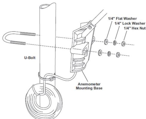
12. Raise the anemometer to the desired height on the pole and swivel it so the anemometer arm is pointing north.
