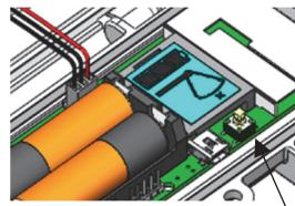
Open the sensor node door and install the rechargeable batteries. Press the button on the sensor node for 3 seconds.
