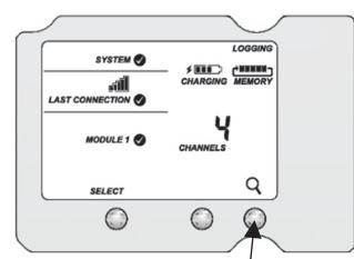
Press the Search button. The magnifying glass icon blinks while the station is in search mode waiting for sensor nodes to join the network.
