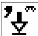
To download the stored readings over **Bluetooth** or USB, click on the download icon. The readings that have previously been recorded will be sent from the Cyclops via USB serial or Bluetooth, along with the extra data associated with each reading. See Appendix 3 for the data stream format.
