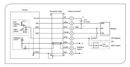
**Power Supply:** Connect the power supply (5 to 27 V DC) to wires 1 (red, +) and 3 (black, Ground)
