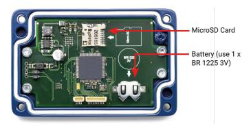
The MicroSD Card and battery slots are located on the touch screen circuit board. Unscrew the lid of the PM030 to access them.
