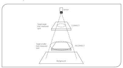
The size of the area (spot size) to be measured determines the distance between the sensor and the target. The spot size must not be larger than the target. Choose a suitable mounting distance so that the measured spot size is smaller than the target.
