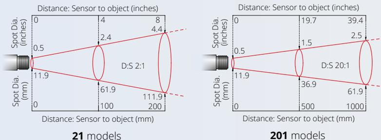
All models can measure at longer distances than shown, with a larger measured spot size.
