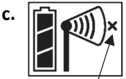
This network connection "x" icon blinks while the repeater completes the registration process, which may take up to five minutes.
