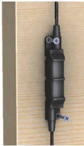
Two Smart Sensor Adapters Stacked and Mounted
